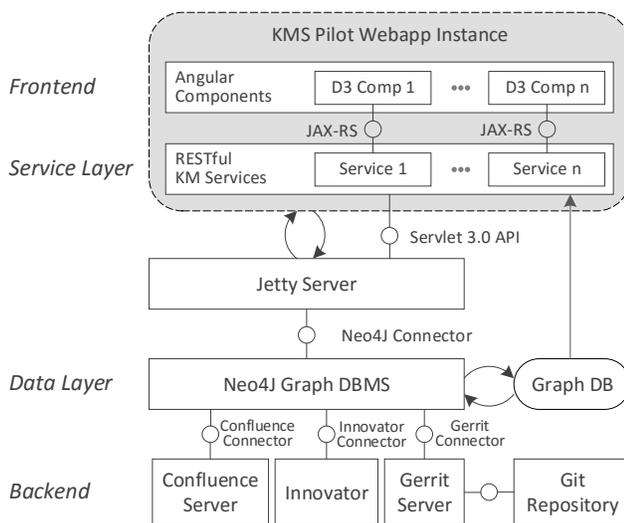
Figure 5: Architecture of the KMS Pilot
